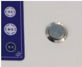
★Note: In "manual mode", it is the start key. When the machine is abnormal, it can be the emergency stop key.
