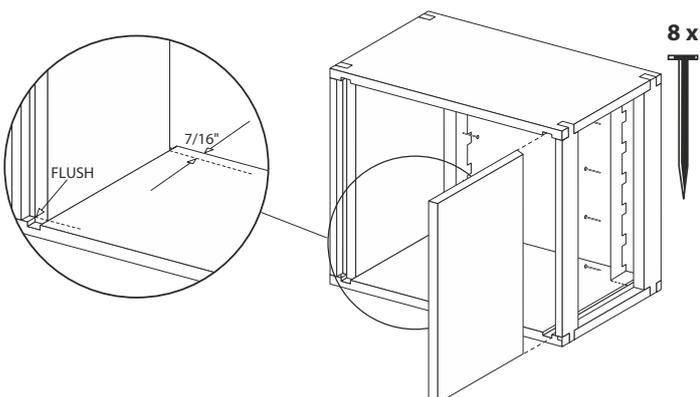
**3** Slide end boards into grooves ensuring chamfered edge is towards top and slopes down and out. The top edge must be 7/16" below the top edge of the side panel. Fit Frame Separators to inside of side panels as shown, using 8 x 19mm frame nails
