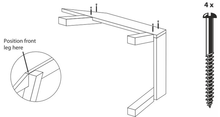
**2** Place left hand side rail and front leg in place as shown and fix using 4 x 40mm black japanned screws.
