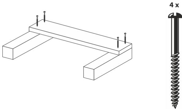
**1** Place rear legs as shown, and fix rear cross rail using 4 x 40mm black japanned screws
