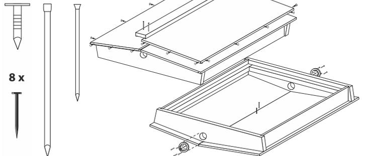
**4** Turn roof over, place metal covers over roof and nail to roof edges using 20 x 12 mm round head nails. Position apex cover strip as shown and nail to roof end boards using 4 x 40 mm lost head nails. Turn roof over and nail through roof panels into apex cover strip using 2 x 25 mm pins. Position vent covers over vent holes and nail in place using 8 x 12 mm black japanned round head tacks.
