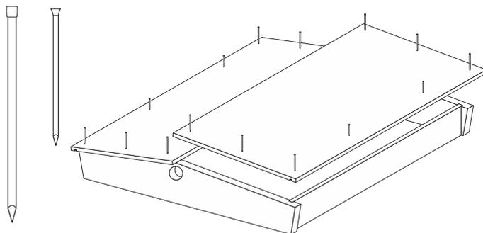
**3** Position roof panels as shown (overhang equally at each end) and nail to end boards using 12 x 40 mm lost head nails. Nail to sides using 4 x 25 mm pins.
