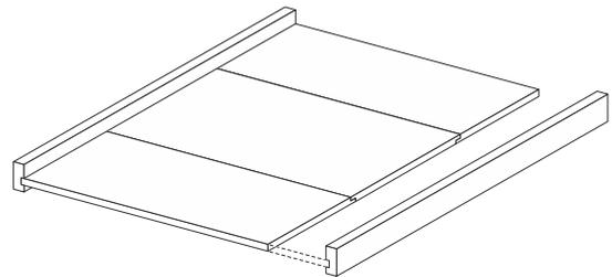
**2** Slot side rails onto floor edges; groove should be to bottom of rail.
