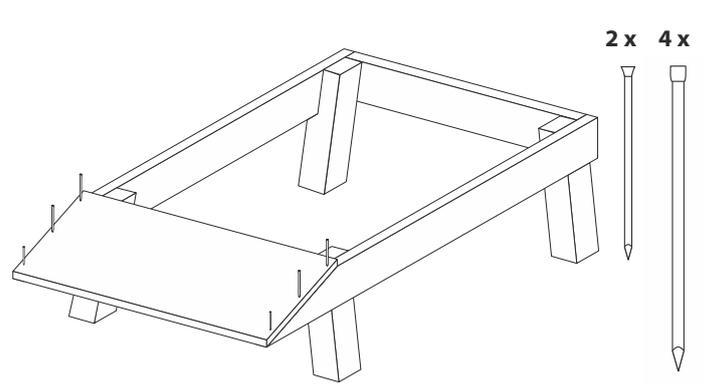
**4** Nail the front slope into place, flush to the front edge of the side rails with its front edge vertical, using 2 x 25mm pins and 4 x 40mm lost head nails
