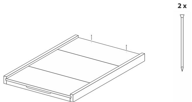
**4** Turn floor over and nail through floor into back block using 2 x 25mm pins.
