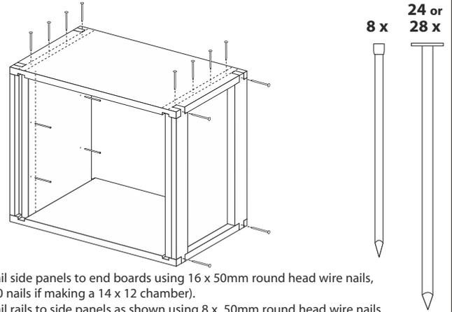
**4** Nail side panels to end boards using 16 x 50mm round head wire nails, (20 nails if making a 14 x 12 chamber). Nail rails to side panels as shown using 8 x 50mm round head wire nails. Nail end boards to rails using 8 x 40mm lost head nails
