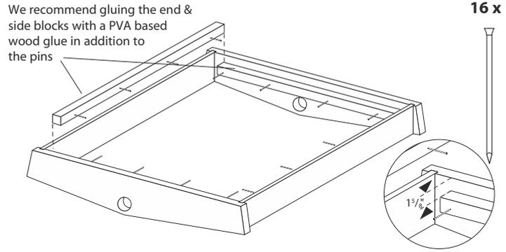
**2** Turn roof over and position inner end blocks and inner side blocks  $1\frac{5}{8}$ " from the lower edge of the roof. Nail to ends and sides using 4 x 25 mm pins per block.
