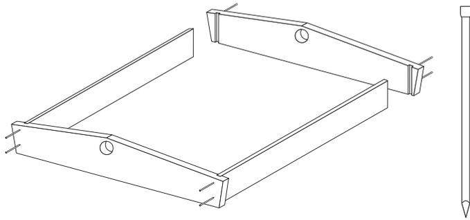
**1** Assemble roof ends to side rails sides as shown. Nail through ends into side rails using 8 x 40 mm lost head nails. Check assembly remains square.
