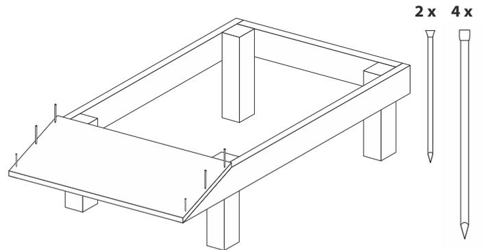
**4** Nail the front slope into place, flush to the front edge of the side rails with its front edge vertical, using 2 x 25mm pins and 4 x 40mm lost head nails
