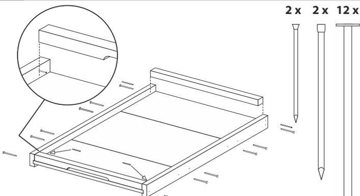
**3** Nail side rails to floor panels using 12 x 50mm round head nails. Position back block between rails and nail using 2 x 40mm pins. Position front/entry block between rails and scribe inner edge to side rails. Remove block and tap in a 25mm pin to half it's length at scribed line to prevent block being pushed into hive. Front block is left loose.
