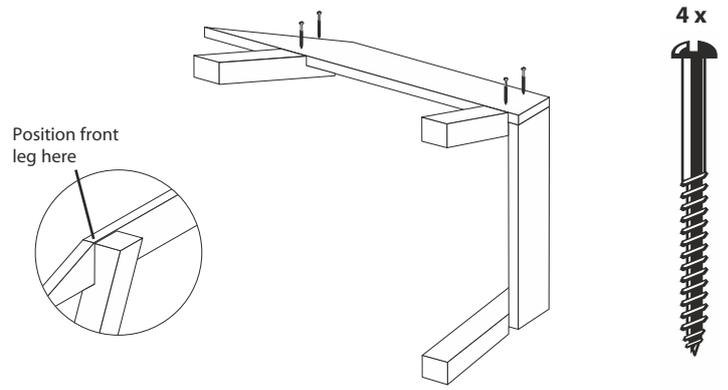
**2** Place left hand side rail and front leg in place as shown and fix using 4 x 40mm black japanned screws.
