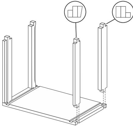
**1** Lay side panel flat. Insert top rails with cutouts facing in and up. Insert bottom rails with chamfer sloping down and outwards.
