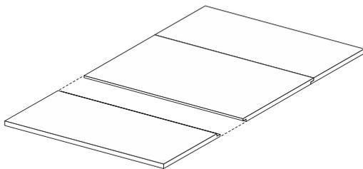
**1** Place floor panels flat fitting rebates together as shown.
