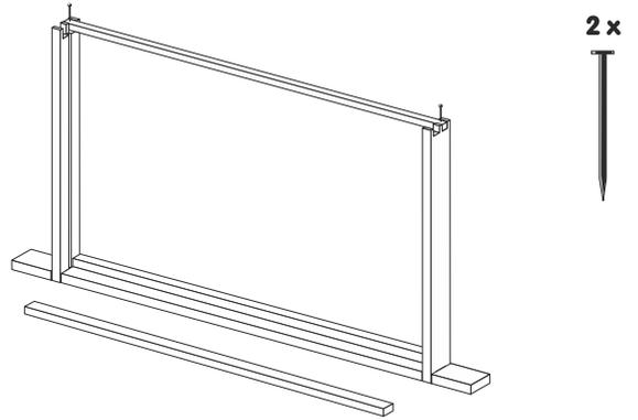
**2** Place first bottom rail in position as shown and nail in place as indicated with 2 x 19mm black Gimp pins.
