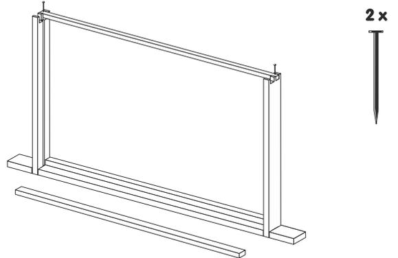
**2** Place first bottom rail in position as shown and nail in place as indicated with 2 x 19mm black Gimp pins.
