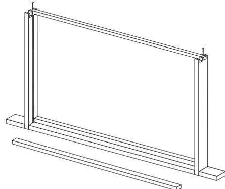
**4** Press wedge strip (from step 1) between side rails, down onto wire loops as shown and nail into rear of top rail with 3 x 19mm black Gimp pins as shown. Fit second bottom rail and nail in place as indicated with 2 x 19mm
