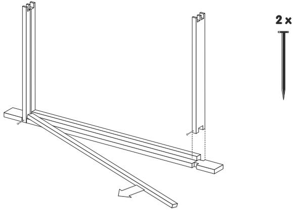
**1** Break out wedge strip from Top bar & retain. Slot side bars onto top bar as shown, with groove to inside. Nail in place as indicated with 2 x 19mm
