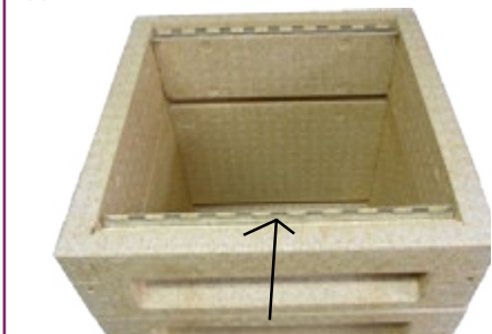
Pic 3. Behind the frame runner is a slot which will accept castellated frame spacers if required.
