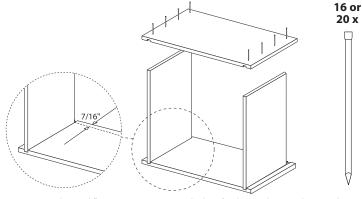
Lay side panel flat. Insert suppport panels chamfer sloping down and outwards into rebates. The top edge must be 7/16" below the top edge of the side panel. Nail side panels to support boards using 16 x 40 mm lost head nails, (20 nails if making a 14 x 12 chamber)
