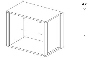
Nail through side panels into side blocks using 4 x 25 mm pins, ensuring side blocks remain flush with lower edge of side strip.
