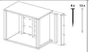
Fit second pair of blocks between side panels and nail side strips to side panels, flush to top edge of side panels, using 12 x 25 mm pins. Fit Frame Separators to inside of side panels as shown, using 8 x 19mm frame nails.
