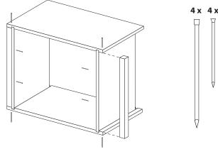
Place side blocks in position, flush to corners as shown and nail in position using 4 x 25 mm pins and 4 x 40 mm lost head nails
