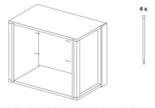
Nail through side panels into side blocks using 4 x 25 mm pins, ensuring side blocks remain flush with lower edge of side strip.
