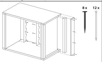
Fit second pair of blocks between side panels and nail side strips to side panels, flush to top edge of side panels, using 12 x 25 mm pins. Fit Frame Separators to inside of side panels as shown, using 8 x 19mm frame nails.
