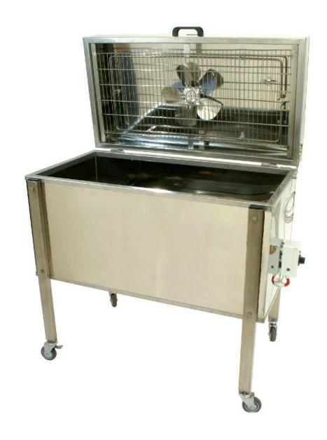
Before the machine is taken into use it is important to ensure that the machine is placed on a stable surface and the wheels are locked in order to keep it from rolling. The machine should be placed in a room with good lightning. This ensures safe and proper handling of the machine. The cord of the machine (230V) is to be placed so it minimises the chance for people stumbling over the cord during operation, cleaning and maintenance work etc.
